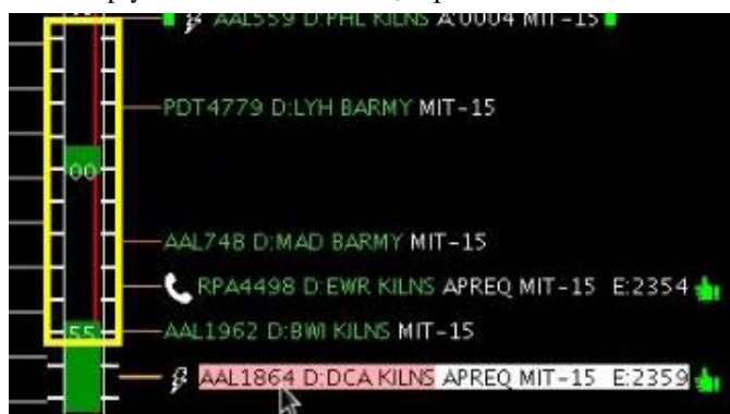
Fig. 3. Slots in the overhead stream for an APREQ flight. (Green slots are available to the APREQ flight, red slots are occupied and unavailable. The yellow box is a visual representation of the EDCT compliance window for the flight..)
